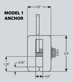
The Model 1 anchor handles seam heights of 1.25" and widths of .6". For illustrations of other models, visit SeamSAFE.com.
