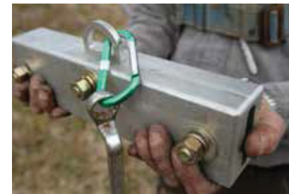
Carabiner shown used for anchor transport only
