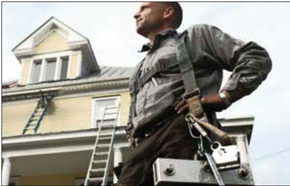
Carabiner shown used for anchor transport only
