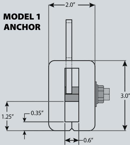
The Model 1 anchor handles seam heights of 1.25" and widths of .6". For illustrations of other models, visit [SeamSAFE.com](http://SeamSAFE.com).
